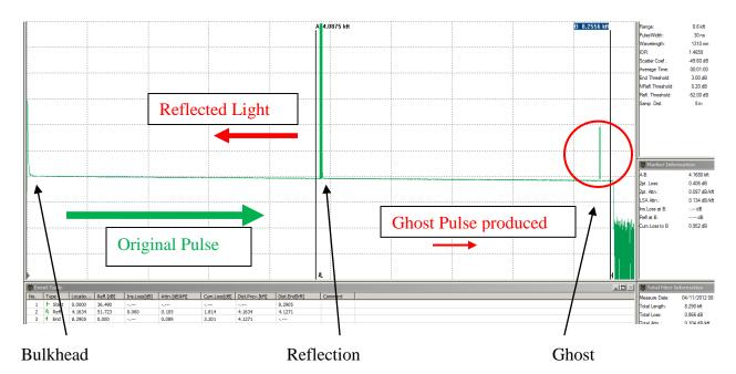
If there was a high reflection at the bulkhead there would be an immediate ghost produced. The effect of ghosting can be reduced if the reflection from the bulkhead is minimized.
