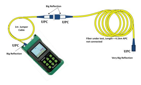
Mated UPC connections have high reflectivity (~45dB) An open (not connected) UPC will have a very high reflectivity (~14dB)
