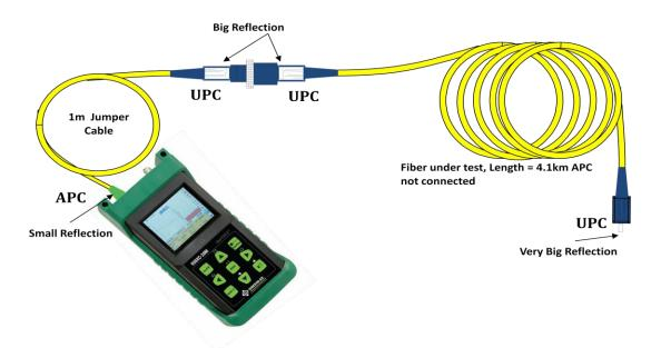
Mated UPC connections have high reflectivity (~45dB) An open (not connected) UPC will have a very high reflectivity (~14dB)
