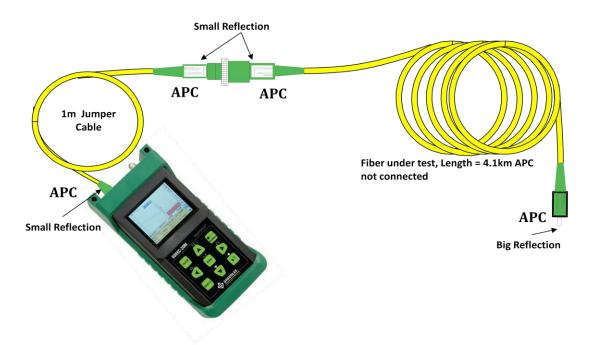
Mated APC connections have very low reflectivity (<65dB typical) An open (not connected) APC will have a high reflectivity (~45dB)
